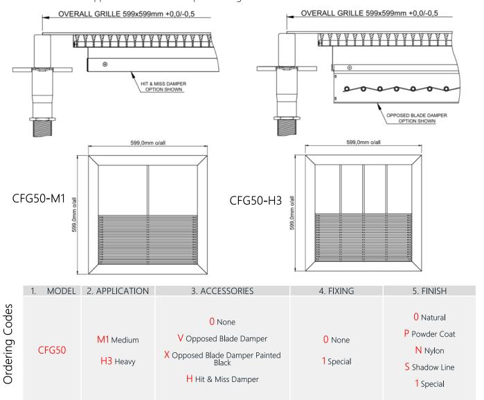
Example: CFG50-H3-H-0-S CFG grille, Heavy Duty, Hit & Miss Damper, No Fixing, Shadow Line
