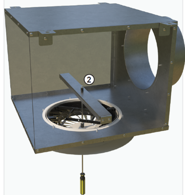
Figure 5 - Installation of a manually adjustable HSC-AD into a plenum box using a central M6 threaded rod ② with decorative cap. Suitable for sizes DN250-DN500 with manual adjustment only.
